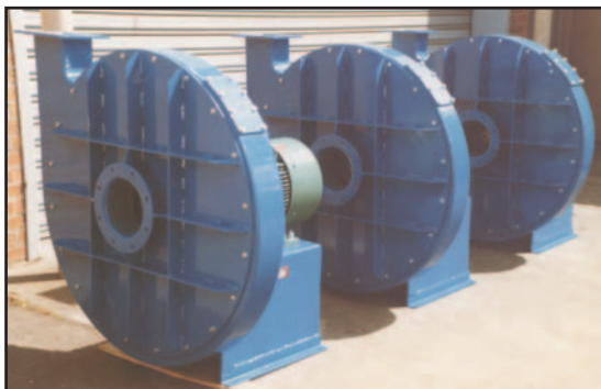
Arr. 4 Direct Driven, Heavy Duty Construction.
